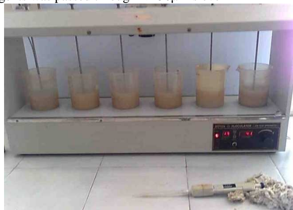
Figure 2. Mixing of chemicals with acid mine drainage
